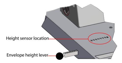
Figure 3-6: Envelope height adjustment
