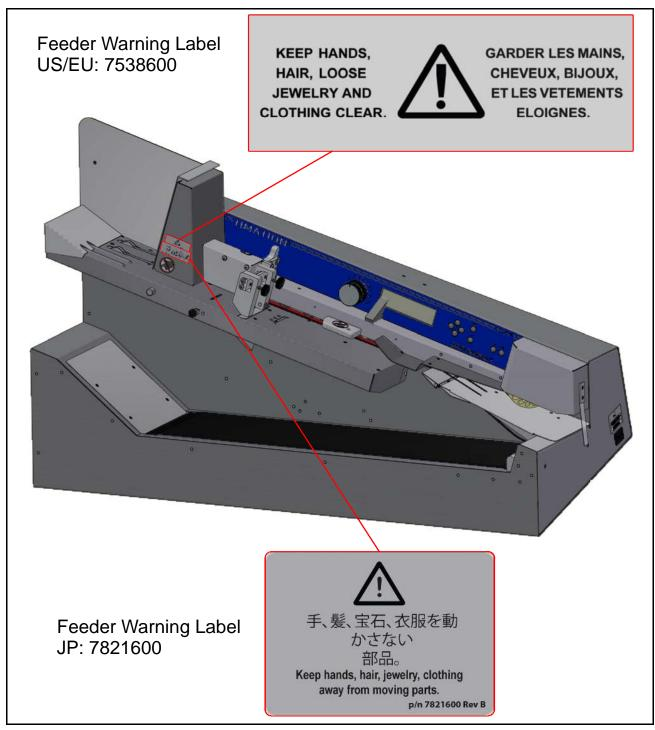
Figure 2-1: Feeder Warning label
