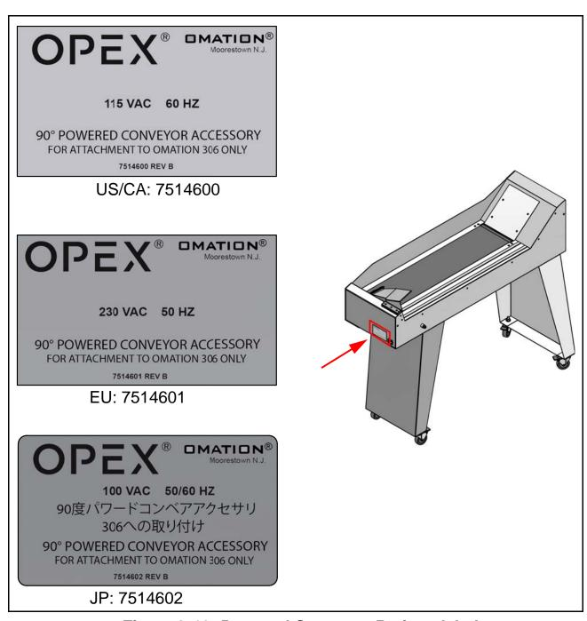
Figure 2-10: Powered Conveyor Ratings label
