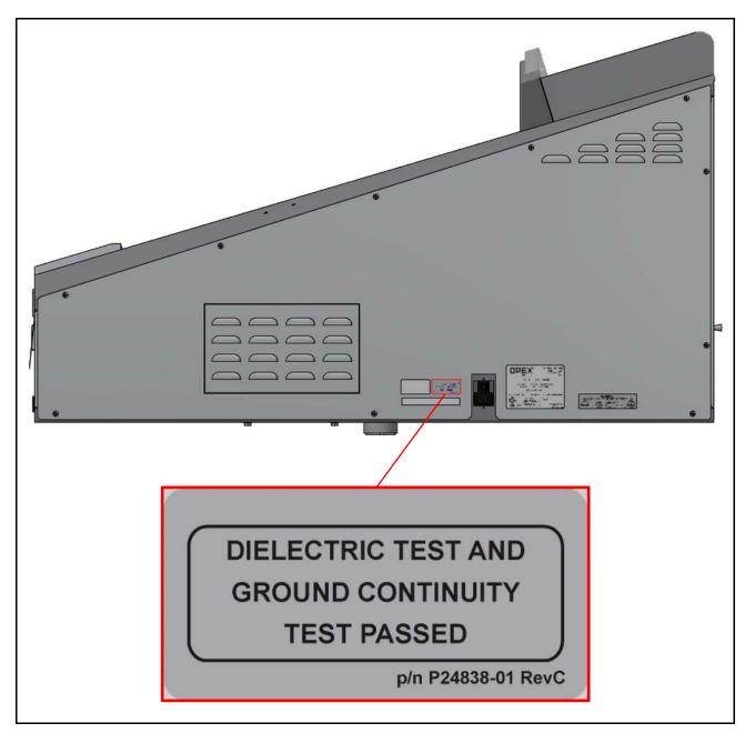
Figure 2-4: Dielectric and Ground Test label 2483801
