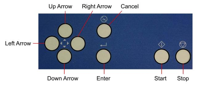
Figure 3-1: Model 306 keypad button names
