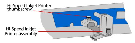
Figure 3-8: Hi-Speed Inkjet Printer adjustment
