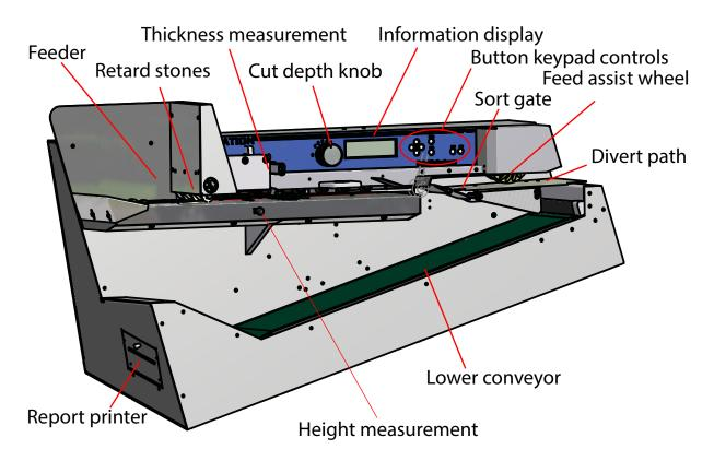
**Feeder** - Envelopes are loaded onto the feeder at the top left of the machine. This area is also often referred to as the hopper.
