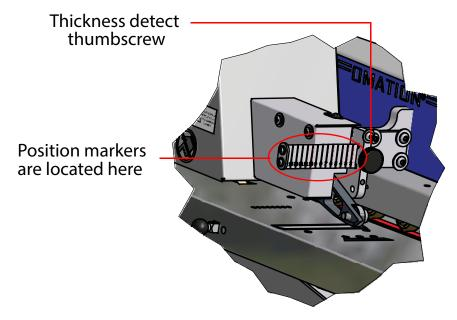
Figure 3-7: Thickness Detect adjustment
